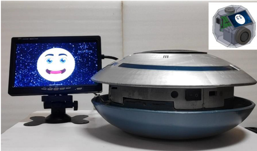
Fig. 3 Voice bot package. Inset is the CAD model of its next version.
